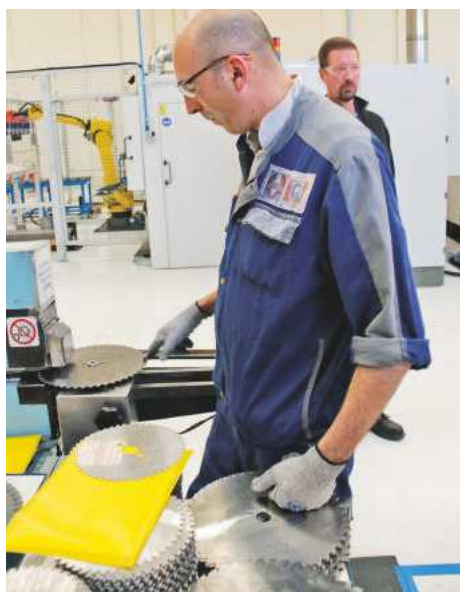
This machine runs a tensioning ring into each blade to keep its tracking true
